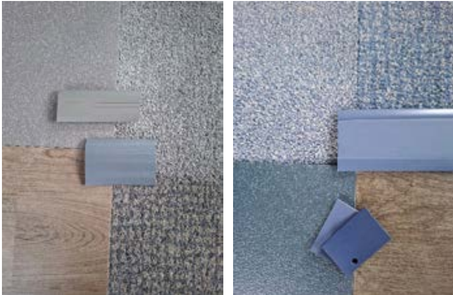
Floor samples selections with low tonal contrast and matching threshold strip. All within recommended LRV variation range. (Courtesy of: DDS Architects)
